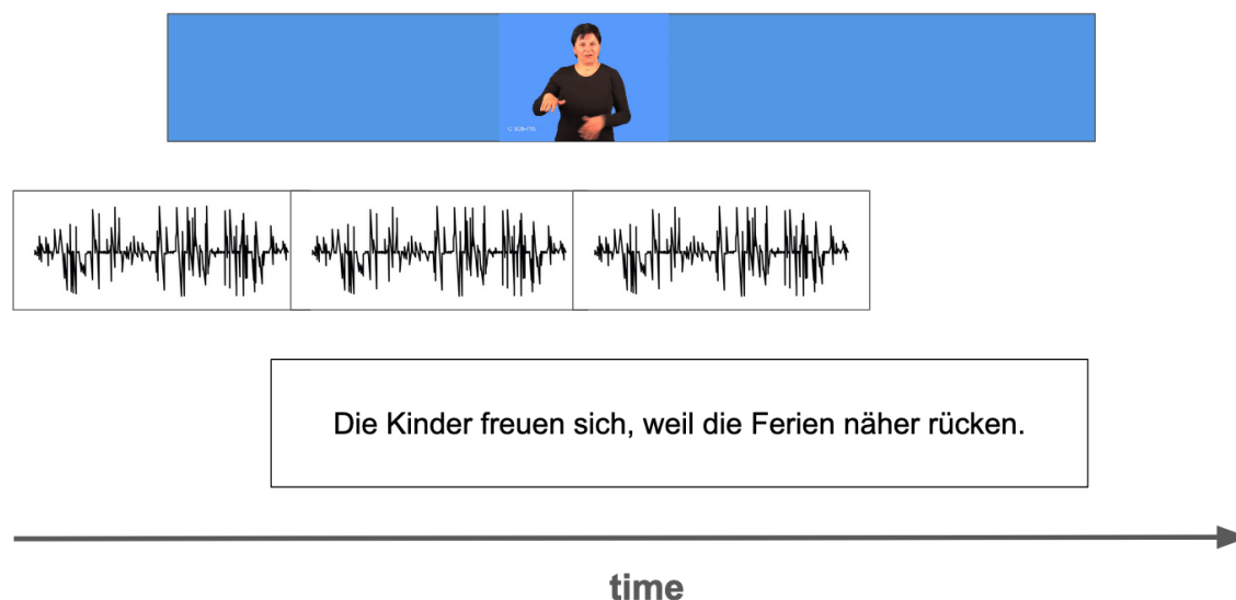
Figure 2.6: Illustration of alignment shift in sign language corpora. From top to bottom: a sign language video, an audio track with speech, a spoken language subtitle in German. Information in these three modalities do not start and end at the same time, adjusting their start and end times is referred to as alignment.
