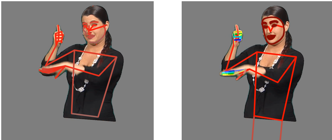
Figure 2.1: Examples of the output of pose estimation systems overlaid over the original video frames. Left: OpenPose, right: MediaPipe Holistic.
